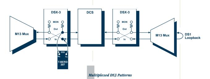
Simulates 3:1 multiplexer or cross-connects for DS3 and DS1 circuit qualification. Test patterns, tones, loop codes, or errors can be inserted on one or all DS1 channels for additional testing flexibility. DS1 channels can be externally analyzed or dropped from the received DS3 signal.
