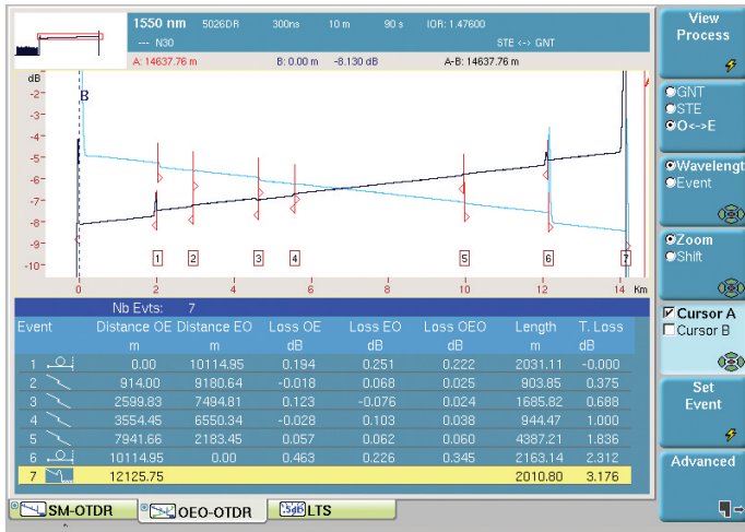
Figure 83. Bidirectional OTDR analysis with the VIAVI T-BERD/MTS platforms
