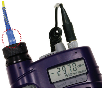
Figure 71. Patch cord inspection
