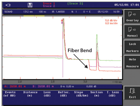
Figure 65. The OTDR graph shows a bend located at 3040 m at 1550 nm and 1625 nm
