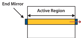
Figure 50. A schematic diagram of a Fabry Perot laser
