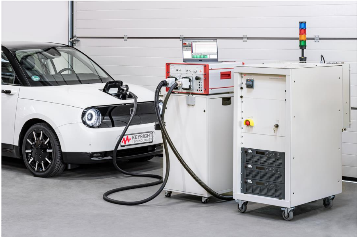
Keysight's SL1202A Scienlab Regenerative AC Emulator (right) with SL1040A Scienlab Charging Discovery System – Portable Series (middle) testing an EV's onboard charger (left).
