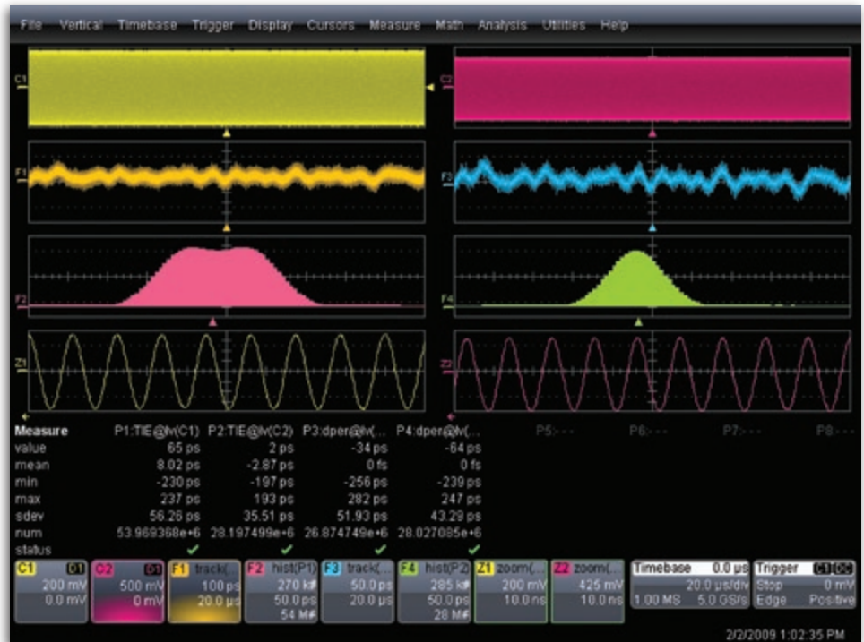
A 200 MHz clock signal is acquired at 10 GS/s using 20 Mpts of acquisition data (400,000 cycles). Cycle-Cycle and Period Jitter are measured and analyzed with Tracks and Histograms. Cycle-Cycle jitter shows a distinctive modality. Other signals could now be acquired and time-correlated to understand the histogram modality.
