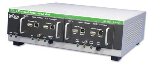
traffic recordings. With interchangeable plug-ins and field upgradeable firmware, the USB *Tracer* analyzer provides both USB 2.0 and OTG support. The OTG support automatically displays host negotiation protocol (HNP) and session request protocol (SRP), and captures Vbus and Data Line pulses allowing for a complete end to end look at OTG occurrences on the bus.
