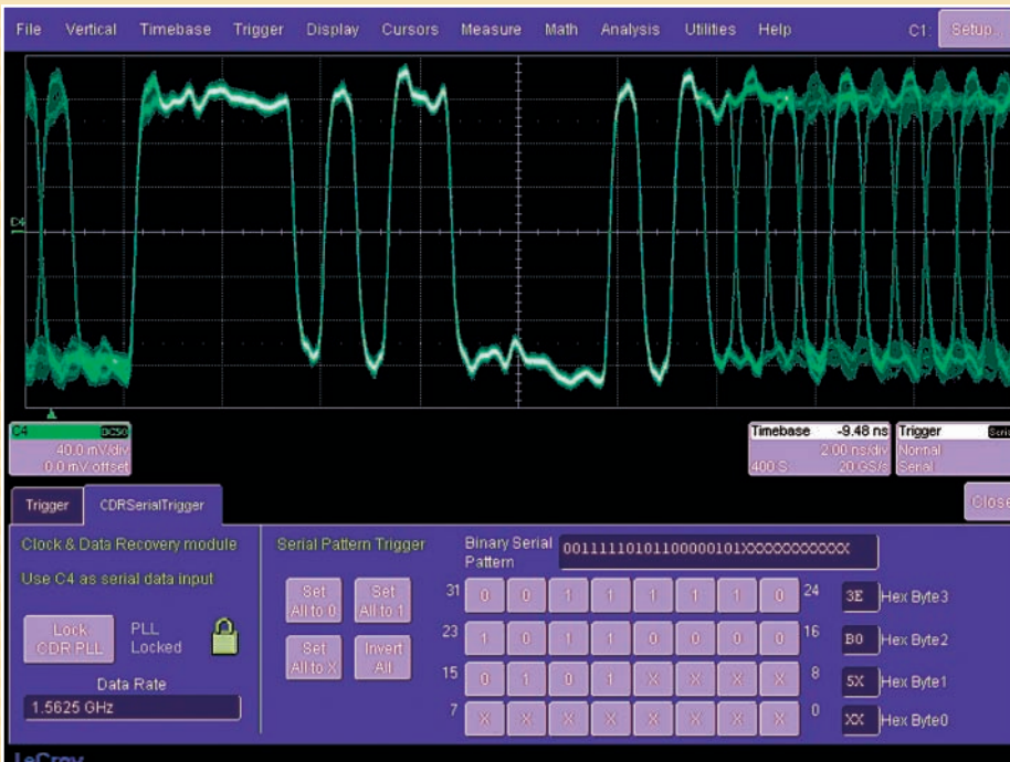
The SDA serial pattern trigger can be used to acquire specific bit patterns for processing.
