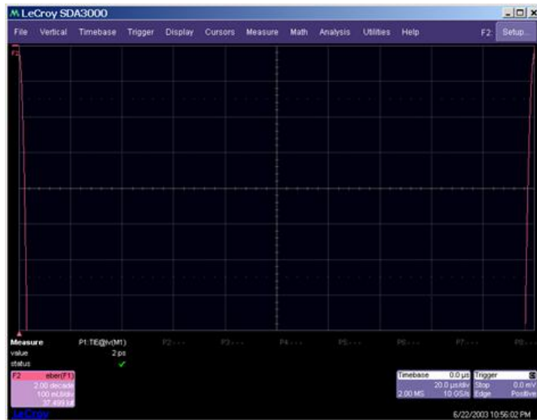
Figure 10. The bathtub curve is constructed by rescaling the total jitter curve in Figure 9 to one unit interval, and centering the right side of the total jitter curve at 0 UI and the left side at 1 UI (the left and
