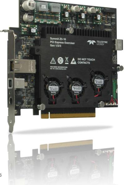
Intuitive software controls blend sophisticated analysis capability with ease-of-use, allowing test suites to be rapidly customized to specific product requirements. One of the many features that helps troubleshoot PCIe<sup>®</sup> links is the ability to exercise LTSSM state transitions.
