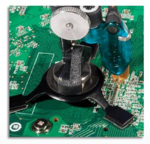
wheel. The probe tips offer a field replaceable pogo pin/spring tip (with a flex of 0.6 mm) to allow robust contact with DUT contacts.
