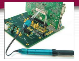
the probe to be used in circuits which cannot drive the low resistance of a pure transmission line probe. The direct cabled SMA inputs have 50  $\Omega$  input impedance with low VSWR.
