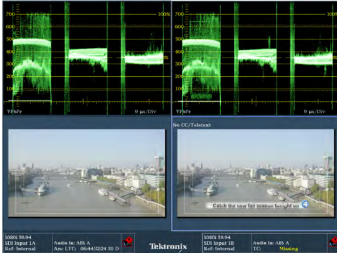
Simultaneous Input mode of WFM7200 comparing incoming and outgoing signals.
