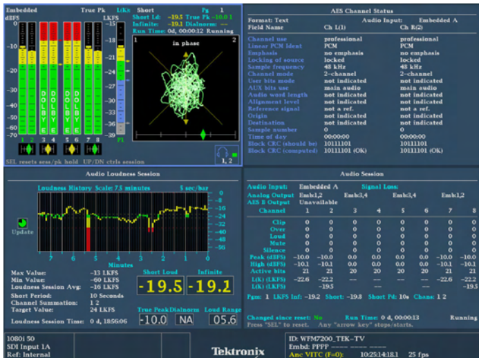
Audio Monitoring with Lissajous display, Channel Status information, Loudness Session, and Audio Session.
