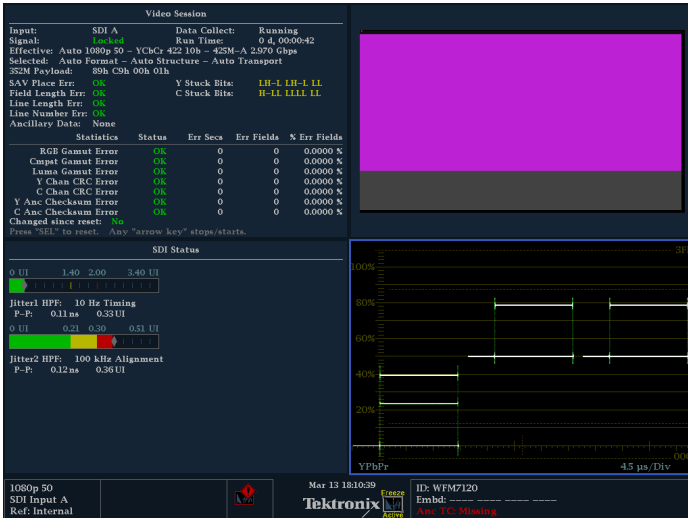
3G Monitoring, jitter measurement, and loop-test generator
