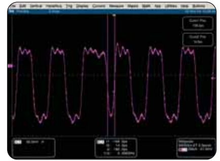
► Trigger on glitches down to 100 ps wide.
