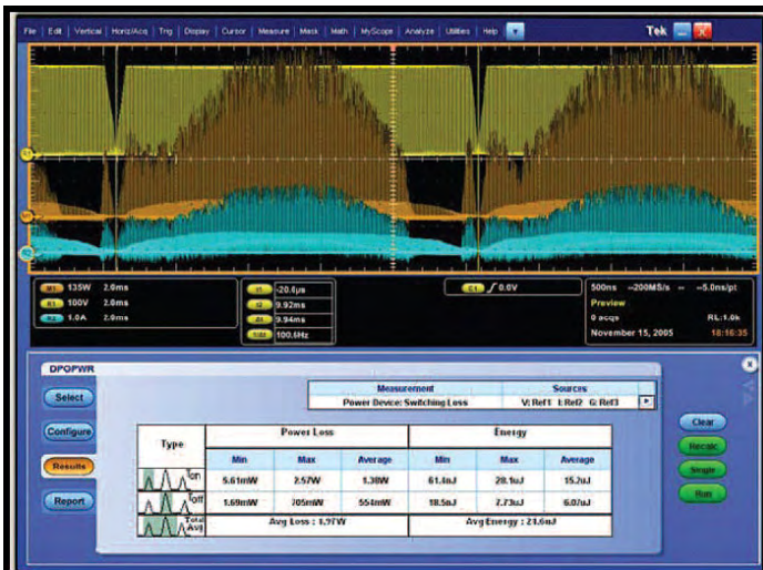
Power Measurement and Analysis Software (Option PWR) – Improve the efficiency of switching power supplies with increased power densities. Measure and analyze power dissipation in power supply switching devices and magnetic components, and generate detailed test reports in customizable formats.
