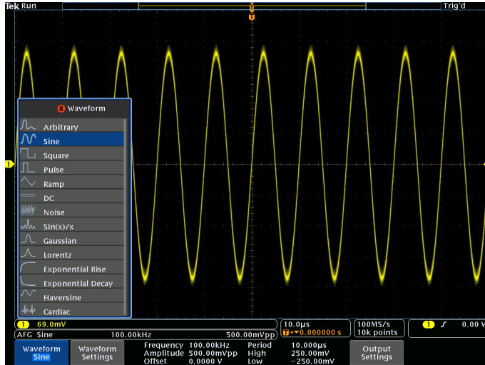
Waveform type selection in the integrated AFG.
