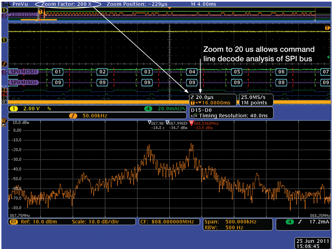
Figure 8. Decoded data and digital waveforms using the Zoom function of the MDO4000 Series Oscilloscope.
