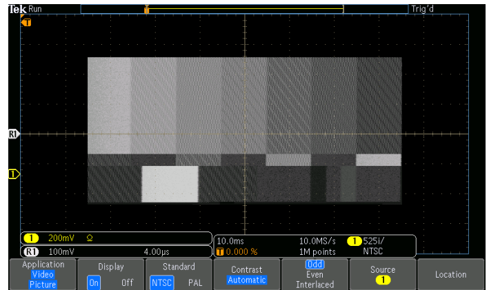
Viewing an NTSC full color bar signal image. Video picture mode contains automatic contrast and brightness settings as well as manual controls.
