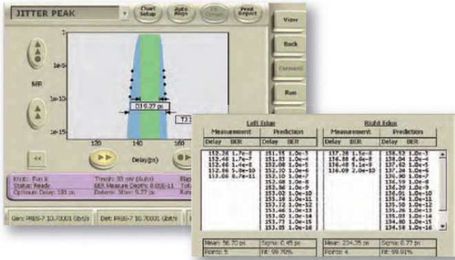
MJSQ-compliant Dual Dirac jitter measurement.
