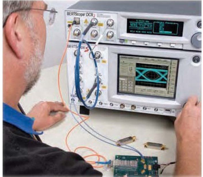
Testing optical transmitters with BERTScope mask testing and a BERTScope CR.
