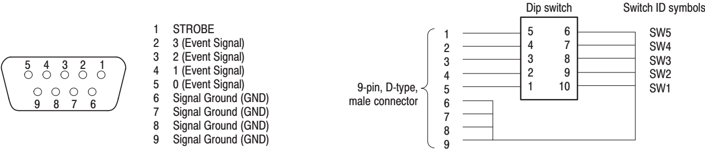
Figure B-3: EVENT IN connector pins and signals and ground closure connector
