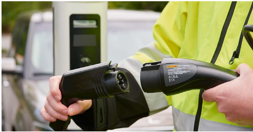
The Fluke FEV100 connects directly to a charging unit to simulate the presence of an electric vehicle.
