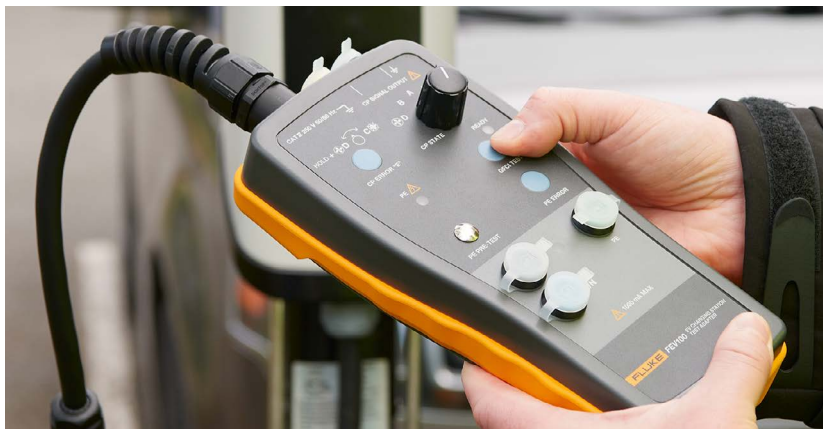
The FEV100 includes a GFCI test function to ensure that the charger's GFCI breaker is working.
