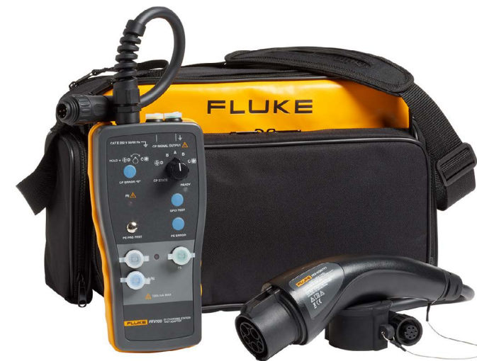
The Fluke FEV100 EVSE Test Adapter simulates the presence of an electric vehicle so technicians can run safety and functionality tests on charging stations without having to connect an EV.
