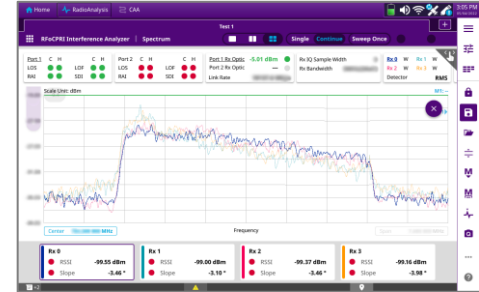
OneAdvisor 800 (RFoCPRITM) PIM Detected: Internal
