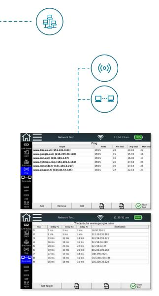
The ping function allows you to check the accessibility of network devices such as servers and printers as well as Internet connectivity.
