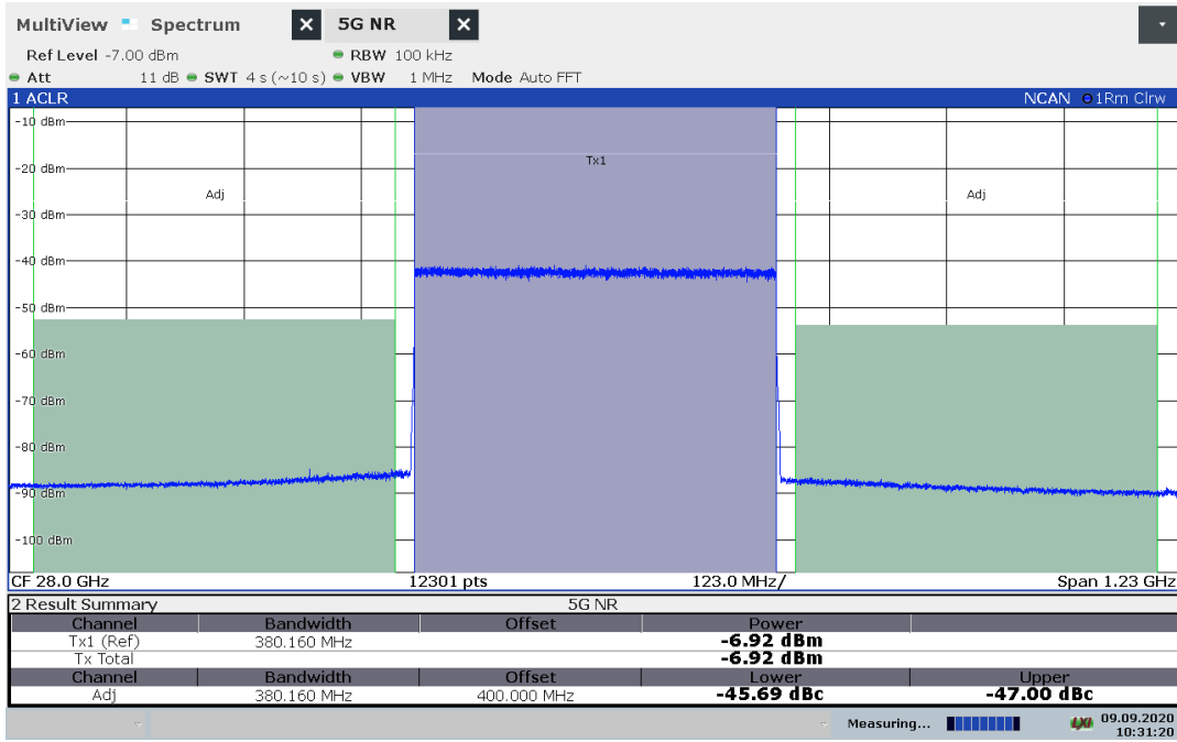
Measured ACPR at 28 GHz for a 5G NR test model NR-FR2-TM3.1; TDD 400 MHz bandwidth, -120 kHz SCS
