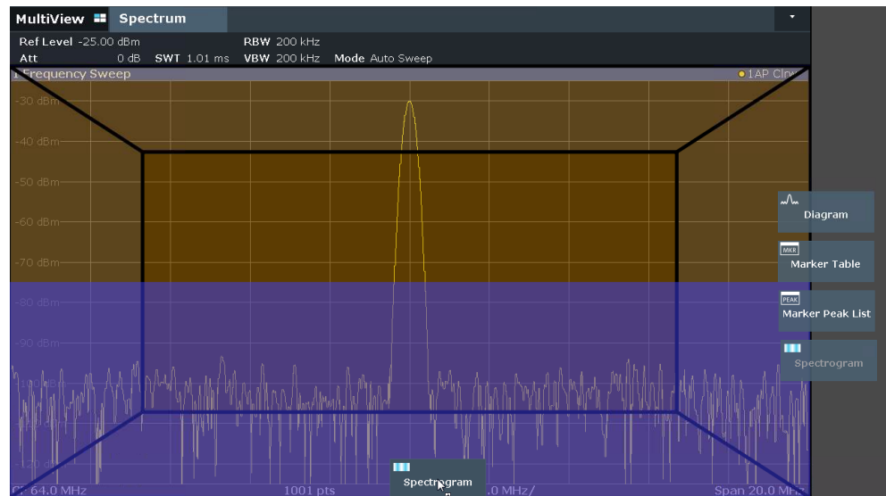
Figure 5-6: Adding a Spectrogram to the display
