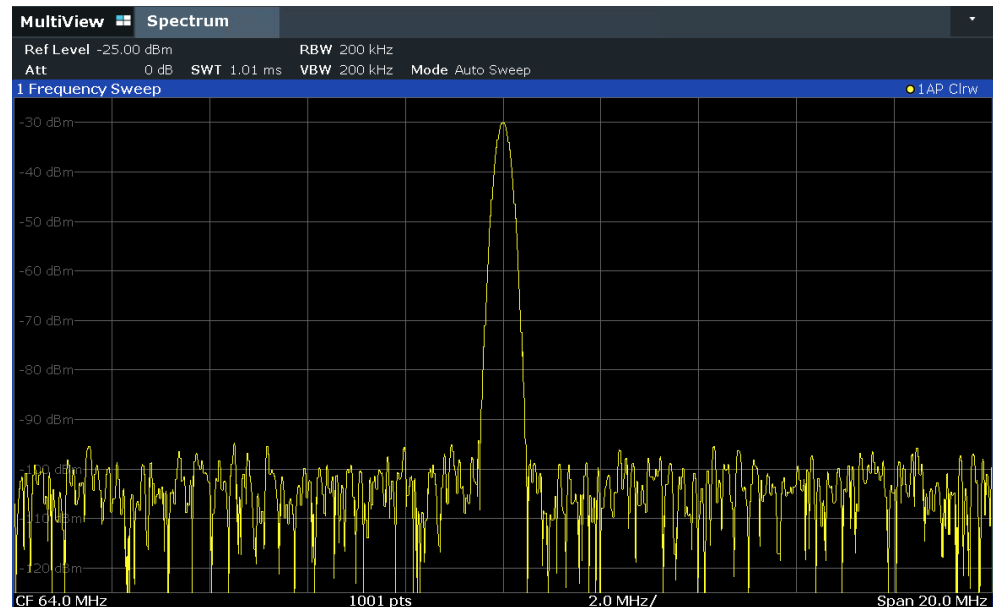
Figure 5-5: Calibration signal with optimized display settings
