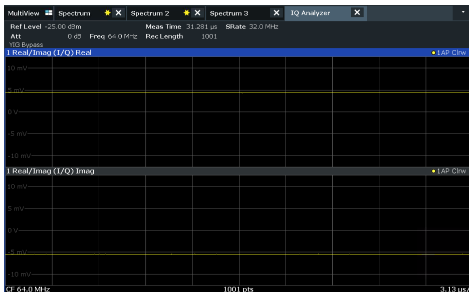
Figure 5-11: Inserting a Real/Imag diagram for I/Q analysis
