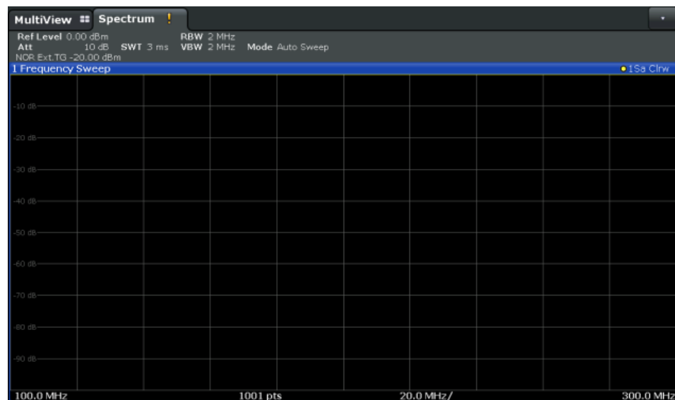
Figure 8-8: Normalized measurement results after calibration
