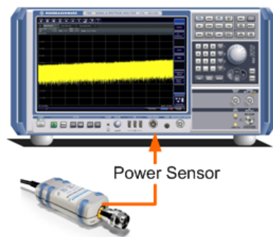
Figure 8-3: Connecting a power sensor using the POWER SENSOR interface
