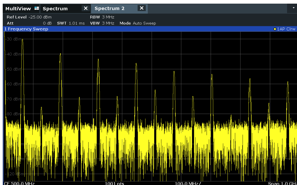
Figure 5-9: Frequency spectrum of the calibration signal with a larger span
