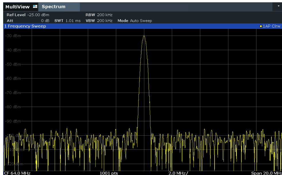
Figure 5-5: Calibration signal with optimized display settings
