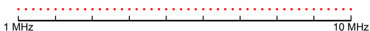
Figure 8-21: Linear x-axis scaling: the distance between the sweep points is equal, e.g. 200 kHz
