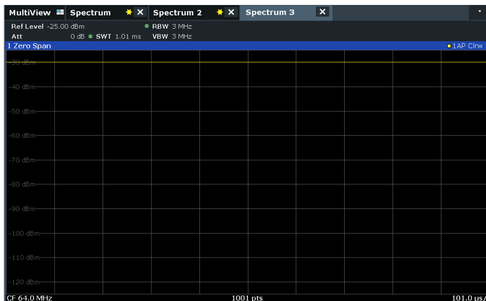
Figure 5-10: Time domain display of the calibration signal
