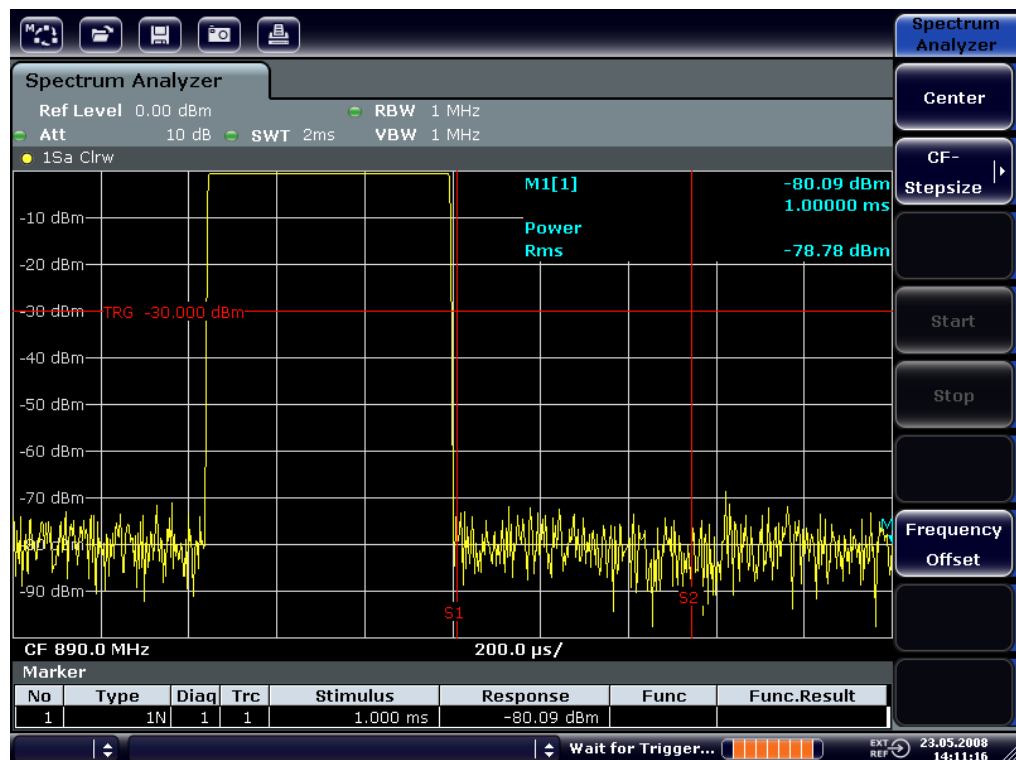
Figure 4-23: Display of the filter edge of the 300 kHz filter as an FM discriminator characteristic
