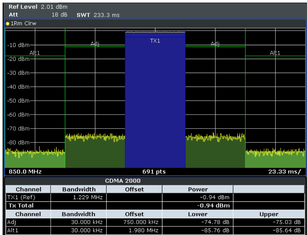
Figure 5-12: Measuring the channel power and adjacent channel power ratio for CDMA2000 1X signals with zero span (Fast ACP)
