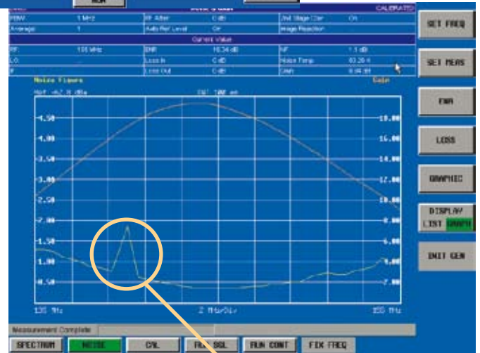
Noise figure measurement using the R&S®FS-K30 Application Firmware.
