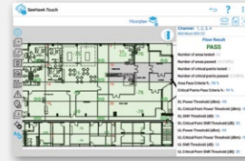
Grid test tool for public safety indoor coverage requirement
