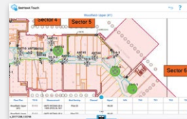
DAS/Small Cell activities antenna verification
