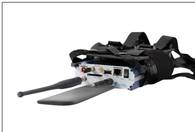
Test setup with antennas connected and scanner in the sidepack
