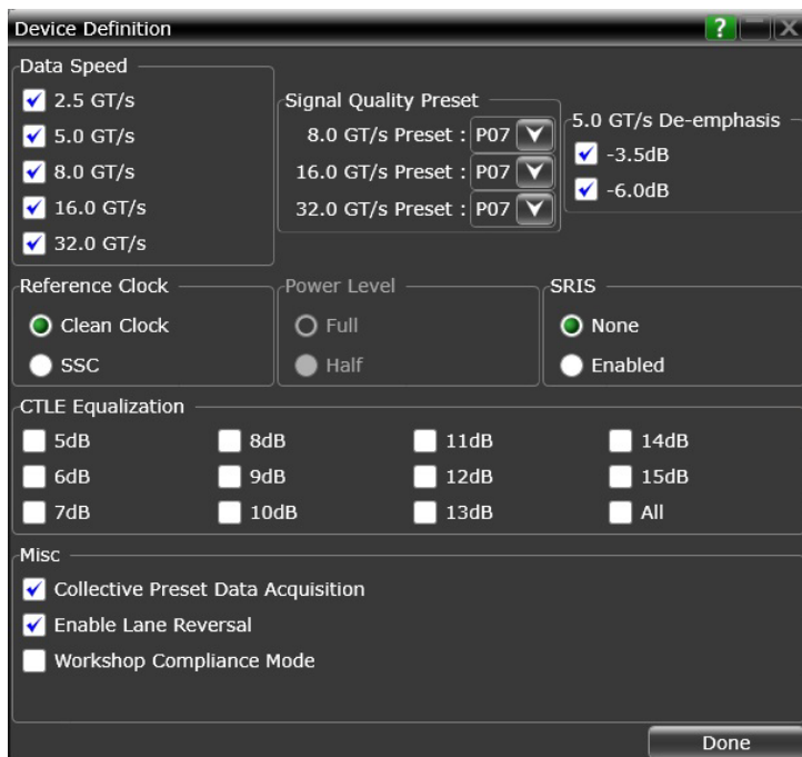
Figure 9: Save TX performance validation test time with the D9050PCIC PCIe test automation software
