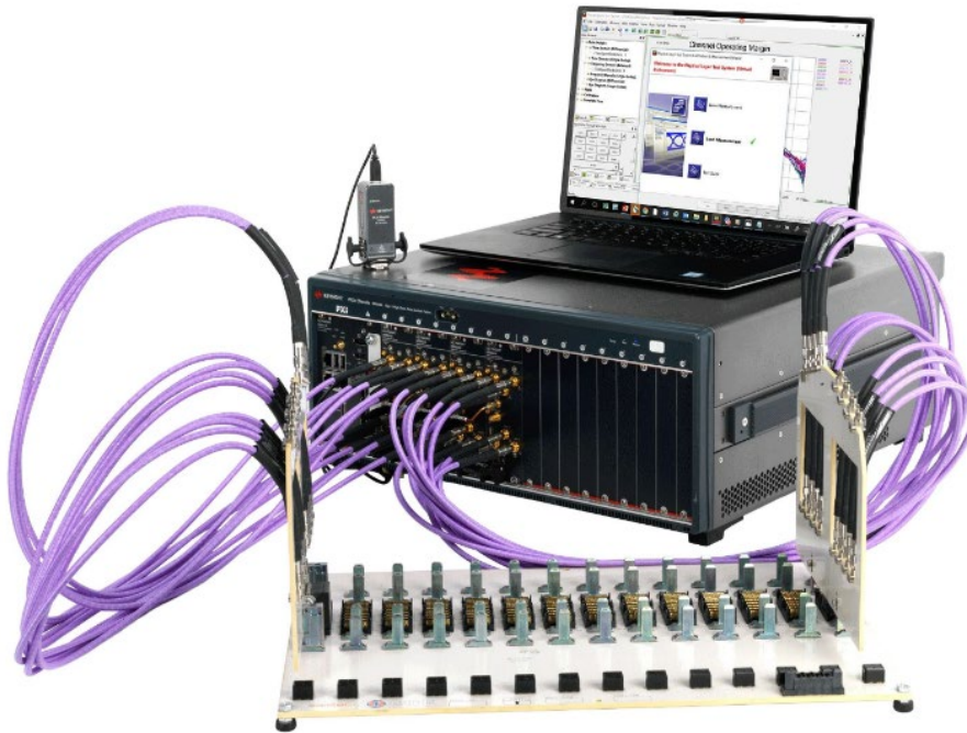
Figure 6: The digital interconnect test system provides full signal integrity characterization of multiport interconnect products.
