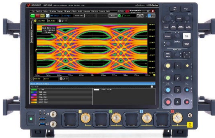
Figure 8: Low-noise UXR real-time oscilloscopes with up to 110 GHz bandwidth for most accurate PCIe TX test
