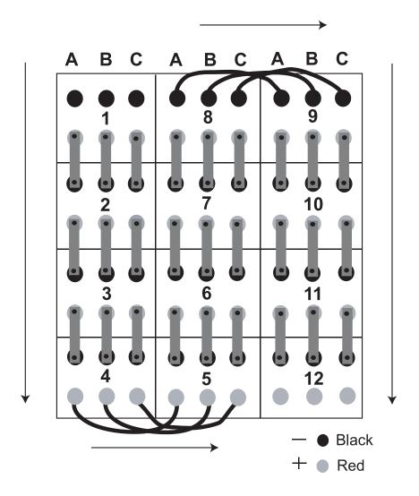
Figure 4: Pattern for testing jars in a string
