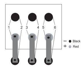
Figure 3: Pattern for testing posts and straps
