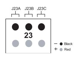
Figure 1: Labels for a jar with 6 posts
