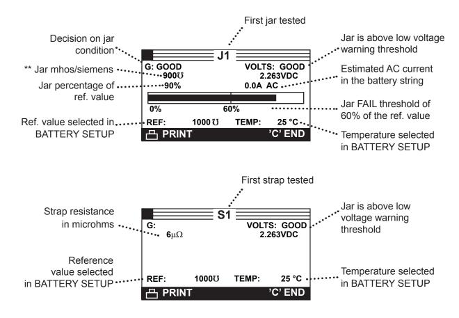
**\*\* NOTE:** The analyzer displays and prints dashes (----) if you selected VOLTS ONLY in BATTERY SETUP, or if you selected VOLTS THEN CONDUCTANCE, but did not complete the conductance measurement.
