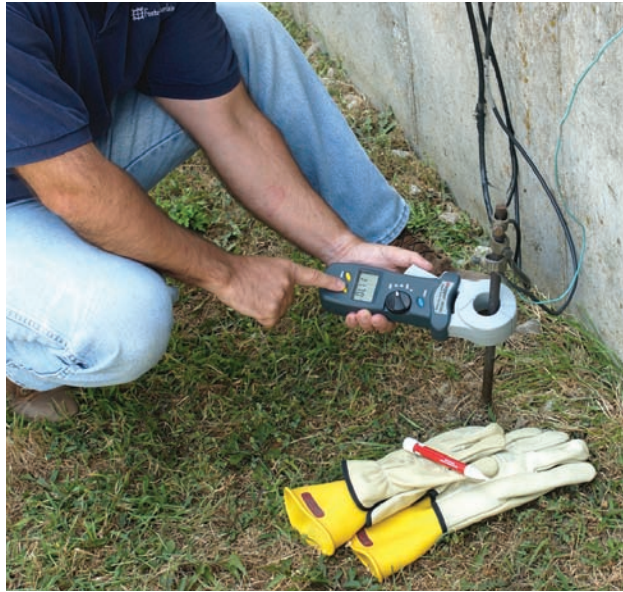
The DET20C instrument is shown being used to test a facility ground.
