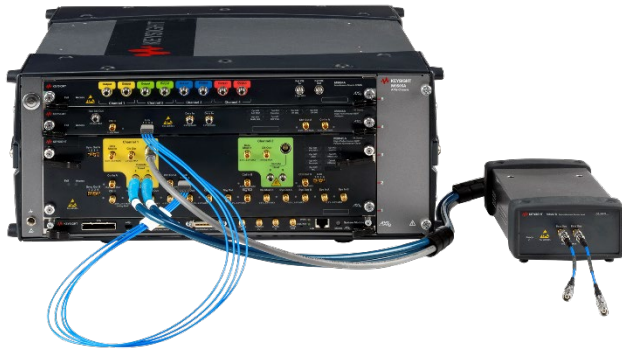
Figure 3. The remote head M8057A/B is required for each channel and is required for NRZ, PAM3 and PAM4 signals. It contains an adjustable gain amplifier without re-timer. Users can select NRZ, PAM3 or PAM4 coding and de-emphasis taps settings from the user interface with no need to reconnect cables. The cable between the remote head and the module is 0.85 m long. This allows positioning the remote head closely to the test board for the device under test.
