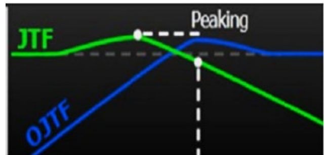
Figure 22. The M8040A provides a built-in- clock recovery option. You can choose between a first and second order PLL characteristic
