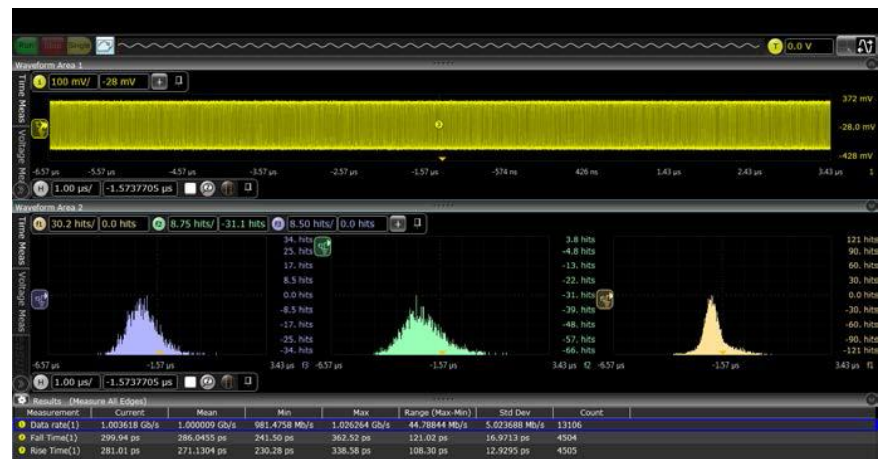
With its flat frequency response and low noise, the UXR-Series is able to accurately measure jitter components such as ISI.
