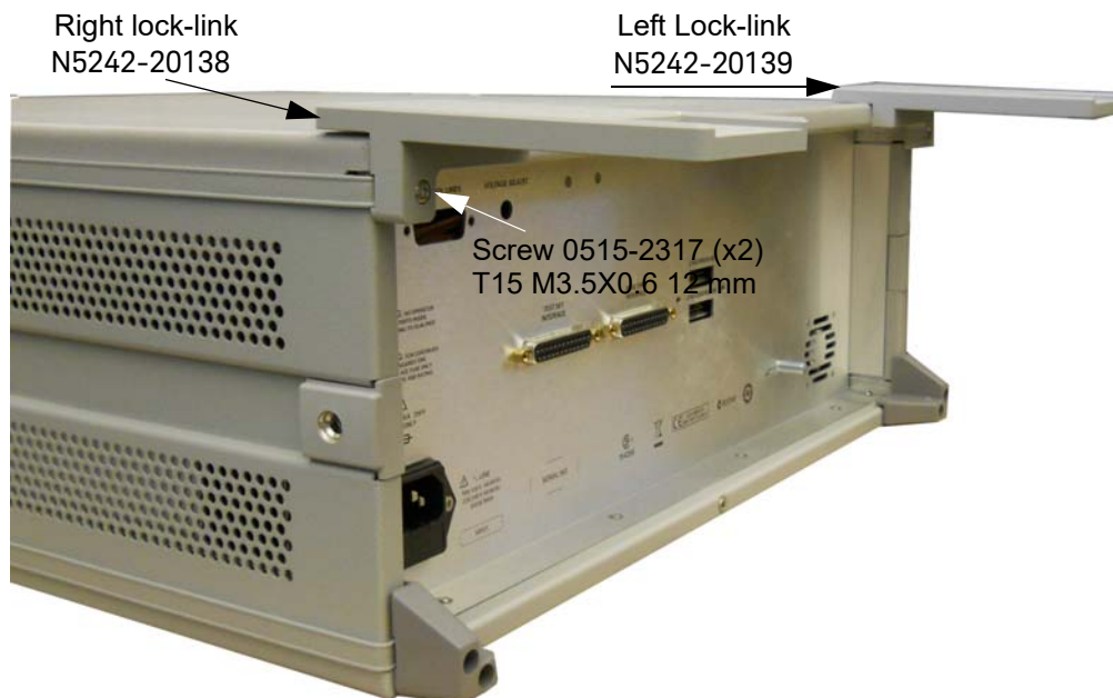
Figure 7 Install Locking Feet on the Test Set
