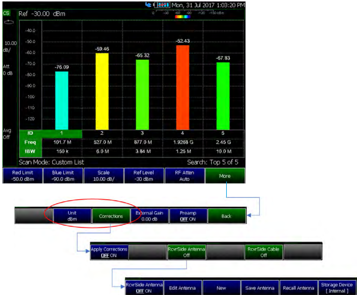
Figure 23-14 Overview of Field Strength for Channel Scanner (See also, Figure 23-15 on page 425 .)
