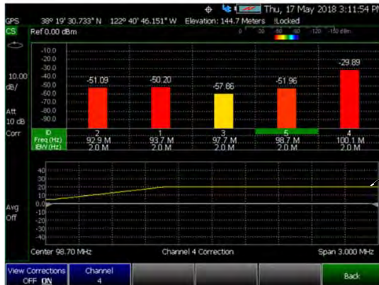
Figure 23-16 Yellow Trace with Cable and Antenna Corrections
