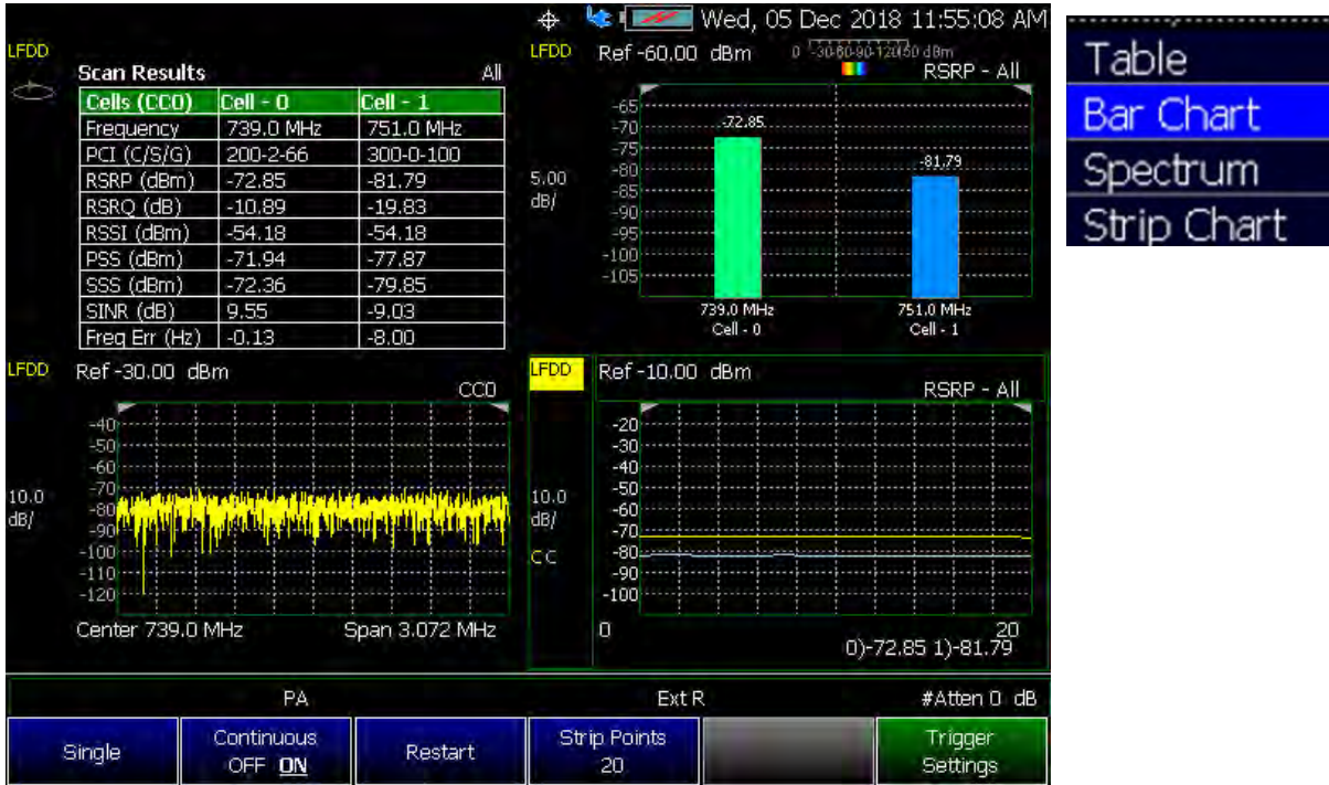
Figure 12-1 Example of the LTE FDD with Four Multiple Display Options
