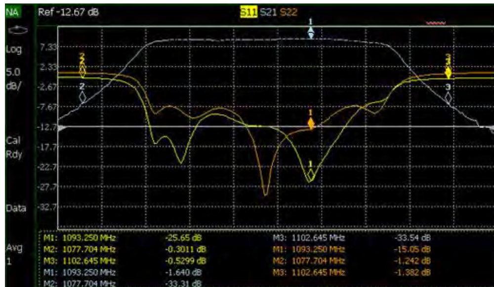
Figure 25-3 Coupled Markers move on ALL traces at the same time (NA shown).
