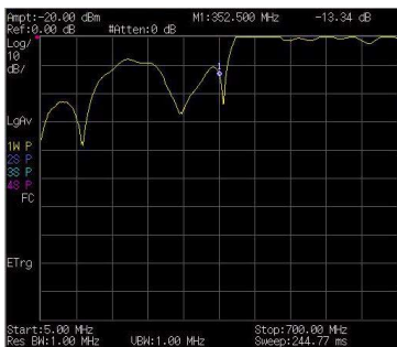
Figure 22 Measuring the Return Loss of the Filter
