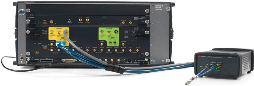
Figure 3. The remote head M8057A is required for each channel and is required for NRZ and PAM-4 signals. It contains an adjustable gain amplifier without re-timer. Users can select NRZ or PAM-4 coding and de-emphasis taps settings from the user interface with no need to reconnect cables. The cable between the remote head and the module is 0.85 m long. This allows positioning the remote head closely to the test board for the device under test.
