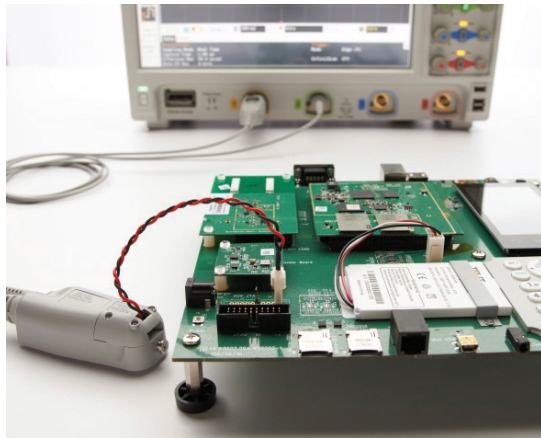
N2820A high-sensitivity 2-channel current probe
