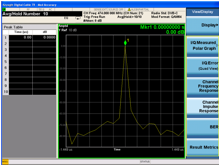
Figure 6. DVB-C channel impulse response view
