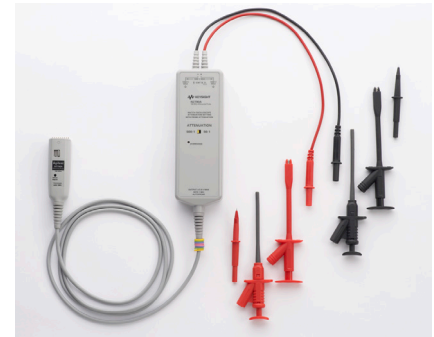
N2790A 100 MHz high voltage differential probe
