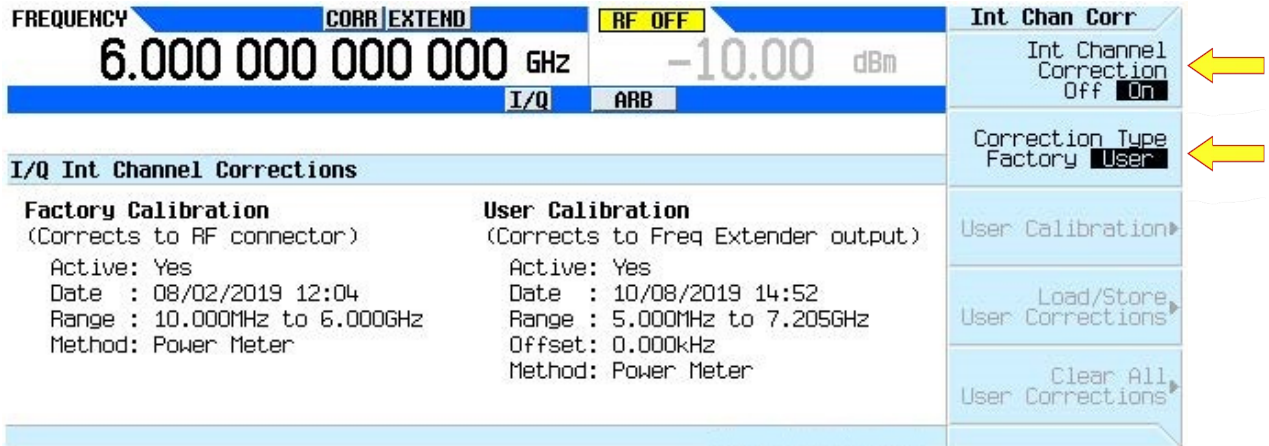
Figure 36 I/Q Internal Channel Corrections
