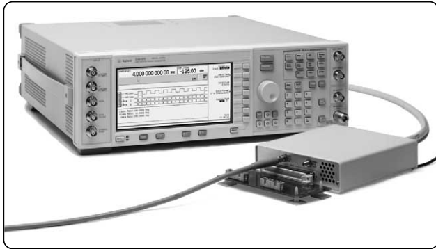
Figure 1. The interface module with the ESG and a single breakout board ready to be connected to a device under test.
