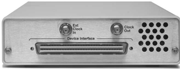
Figure 3. Rear panel clock connectors. Clock the interface module through the device interface bus or the external clock input port. Take the output clock signal from the device interface bus or from the clock output port.
