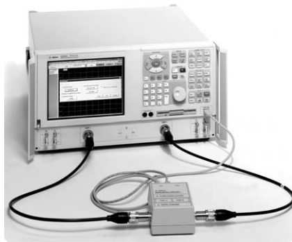
Calibration configuration using the PNA series
