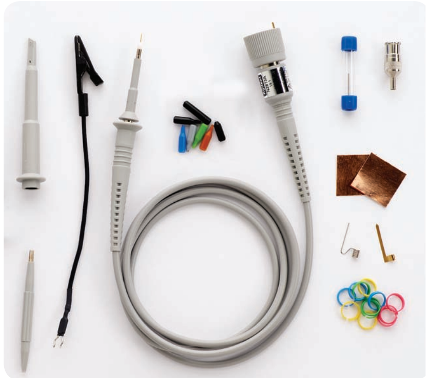
Figure 1. N2873A 500 MHz passive probe with standard accessories
