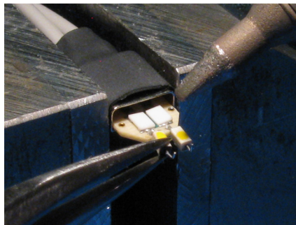
Figure 50 Removing the Resistor
