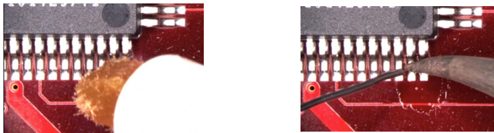
Figure 24 Preparing the DUT Leads
