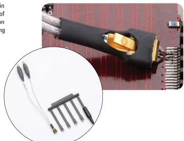
N5444A 2.92 mm/3.5 mm/SMA probe head (28 GHz) allows you to connect two 2.92 mm, 3.5 mm or SMA cables to make a differential measurement on a single oscilloscope channel. Order N5448A 2.92 mm head flex cables (10" or 25 cm) to extend the cable length and add convenience.
