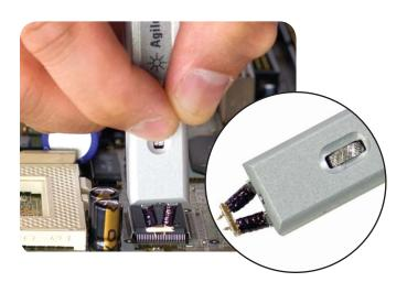
• N5439A ZIF probe head provides 28 GHz bandwidth in an economical replaceable tip form factor. Because of their extremely low loading, the ZIF tips can be left on the DUT as the probe head is moved from one probing site to the next. Order N5440A (450  $\Omega$ ) or N5447A (200  $\Omega$ ) for a set of 5 ZIF tips with plastic sporks to aid in soldering the tips to your DUT. Variable spacing from 5 mil - 80 mil (or 0.127 mm - 2 mm).
