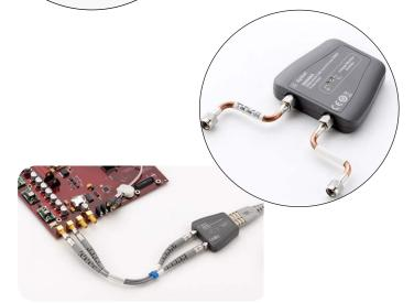
N5441A solder-in probe head is an economical, semipermanent connection that provides up to 16 GHz of bandwidth. Variable span of the leads ranges from 5 mil – 80 mil (or 0.127 mm – 2 mm).
