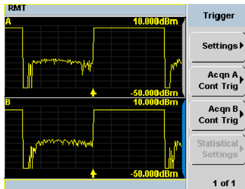
Figure 4-5 Trace display in dual channel power meter
