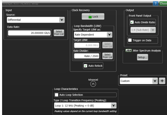
Figure 10. Easily configure the N107x clock recovery data rate, loop bandwidth, and peaking using the N1010A FlexDCA user interface running on an 86100D DCA-X mainframe or standalone PC.
